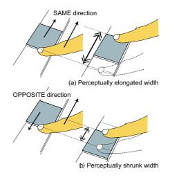
Figure 1: Conceptual figure of display principle.
